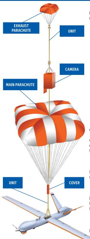
The rescue parachute system SPS-12 / SPS-23 is intended for use safely back of UAV for such methods as "parachute" or emergency landing of the UAV.
