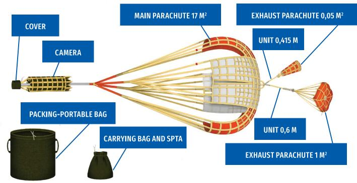
The system provides speed suppression of an aircraft during landing and is deployed at velocity not less than 180 km/h and up to 300 km/h.
